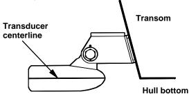
Align transducer centerline with hull bottom.
